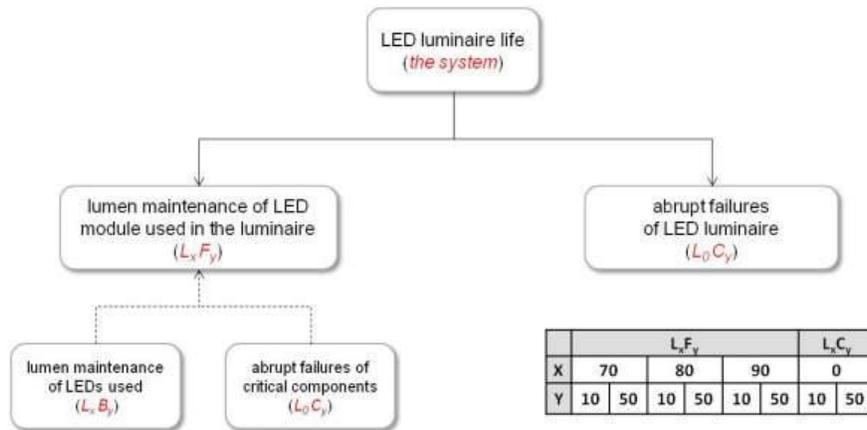
Figure 1: LED luminaire life according to IEC
